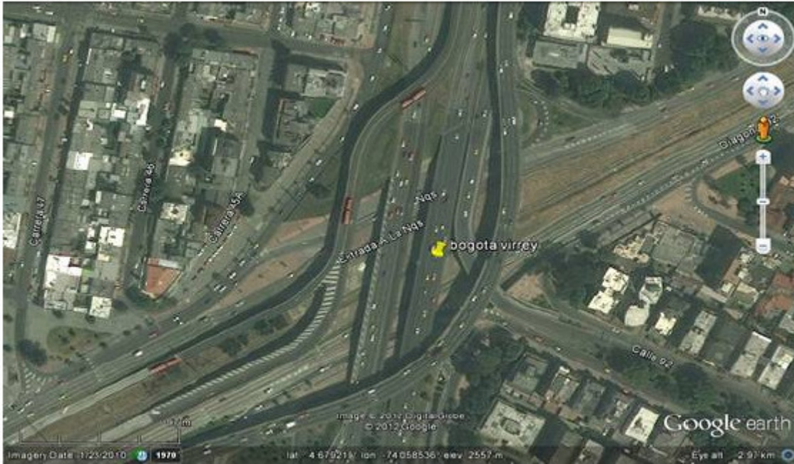
Pic 2. The width of Bogota's freeways and boulevards can be further judged by this satellite view from Google Earth at 4.679219N 74.058536W near bus station Virrey. At this intersection of BRT Routes B and E multi level grade separated flyovers can be seen
